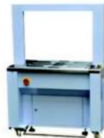
SPS-12.1 PLC Controlled Fully Automatic Strapping Machine (With Japanese Technology) Strapping Speed 1.8sec./strap Packing Size Any Type Strap Size 8-15mm Strapping Tension 48-700N Adjustable
