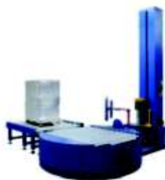
SPS-YK2000FZ-PL Online Pallet Wrapping Machine With Conveyor Wrapping Size 500-1200(L)x500-1200(W)mm Turn Table Weight Capacity 2000kg Turn Table Speed 0-12rpm Turn Table Height 550mm
