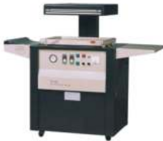
SPS-022 Blister / Skin Packing Machine Packing Area 390x540mm Packing speed 50-60 Pcs/hour Film Width 450mm Packing Material Skin Packing Film
