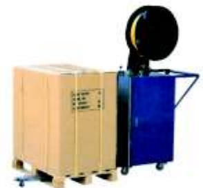
SPS-DBA-130A Pallet Strapping Machine (Standard Style) Strapping Speed 2.0sec./strap Strap Size 9-15mm Strapping Tension 100-700N (adjustable) (For PP Strapping for Pallets)
